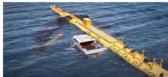
Figure 12: The Orbital O2 (2 MW) tidal turbine by Orbital Marine Power (ex Scotrenewables) [16]
