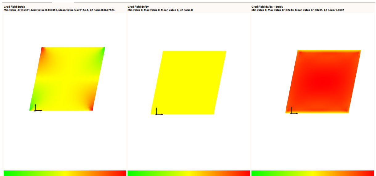
Figure C.20: The displacement gradient fields after a simple shear stretch (two opposite boundaries moved by a unit in opposite directions) of the square domain with size 9 \times 9 . Adaptation with the 0-degree MLS method and an optimized interpolation parameter a .
