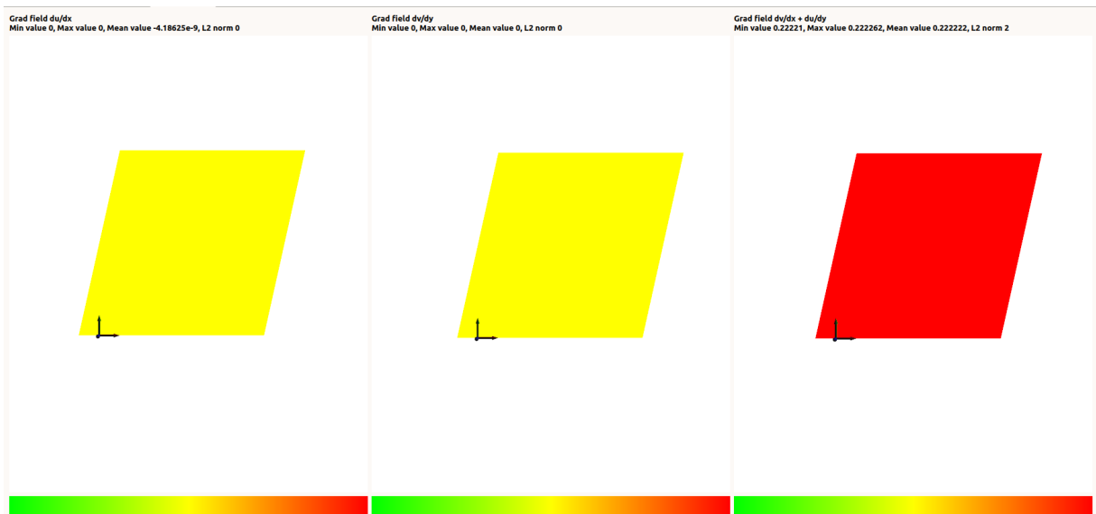
Figure C.19: The displacement gradient fields after a simple shear stretch of the square domain with size 9x9. Adaptation with the 1 st degree MLS method and an optimized interpolation parameter a .
