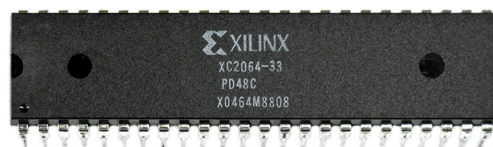
Figure 2.2: The first commercially viable field-programmable gate array in 1985 – the XC2064 † .
