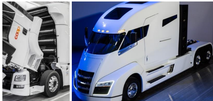
Figure 2-13: ESOROS' truck hydrogen tanks, located behind the cab (left) and Nikola One (right)
