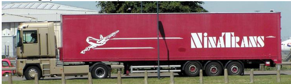
Figure 2-12 Error! Reference source not found. The trailer in this example is called a semi-trailer because there is no front axle attached; instead the rear axle of the truck is used in its place [30].
