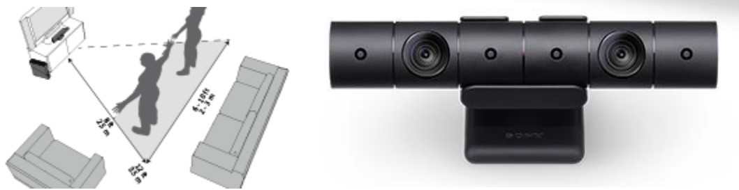
Figure 2: Commercial Visual Based MoCap Products: Microsoft X-BOX Kinect™ 1 (left), SONY PlayStation Camera™ 2 (right)
