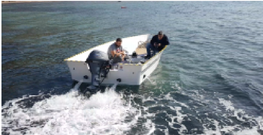
Figure 6.26: Test boat sea trial with transom nozzles enabled
