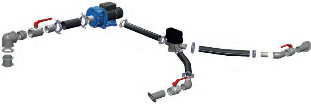
Figure 4.2: Exploded diagram of Jet-Thruster JT-30 compact system
