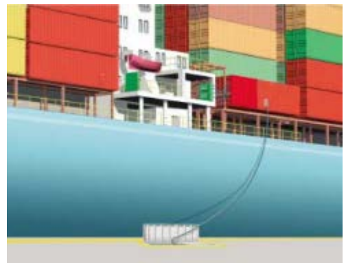
Figure 2.7: Mobile ship-based cable management system
