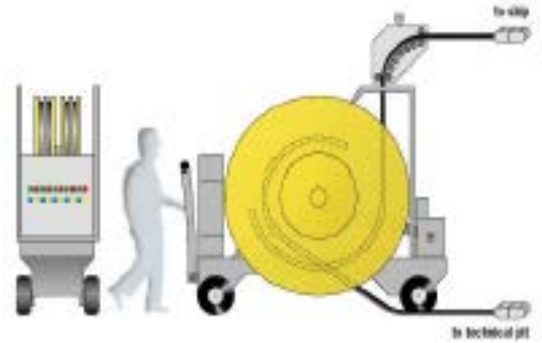
Figure 2.5: Mobile shore-based cable management system
