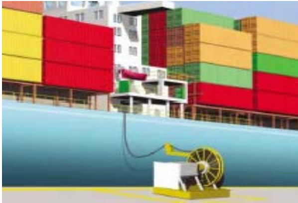
Figure 2.4: Fixed shore-based cable management system
