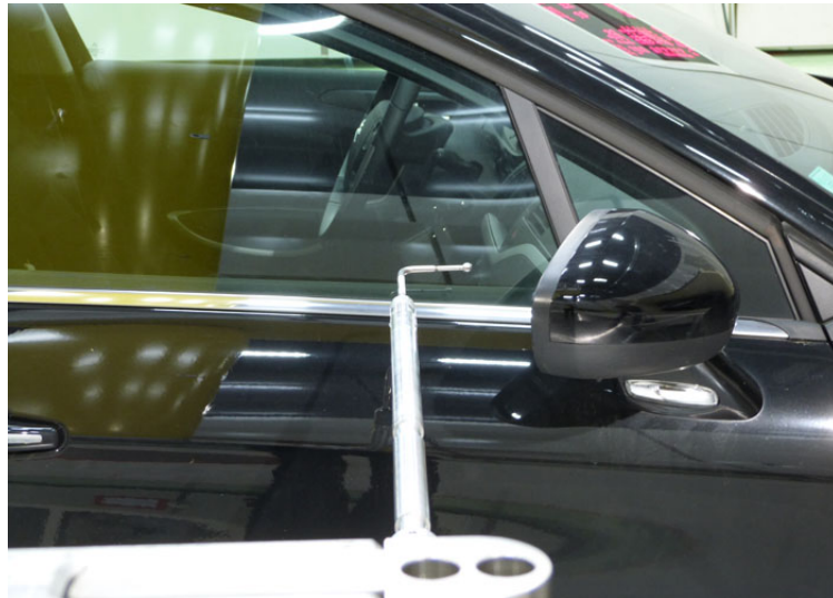
Figure 4.36: Application to a Production Car. The L-shaped 18 hole omnidirectional probe used to measure the mirror's wake. From [35].
