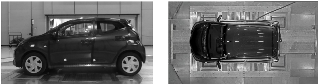
Figure A.2: The two planes available for noise source localization; side plane A1(left) and top plane A2(right).
