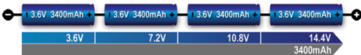
FIGURE 2.4: Series connection of four cells (4s).
