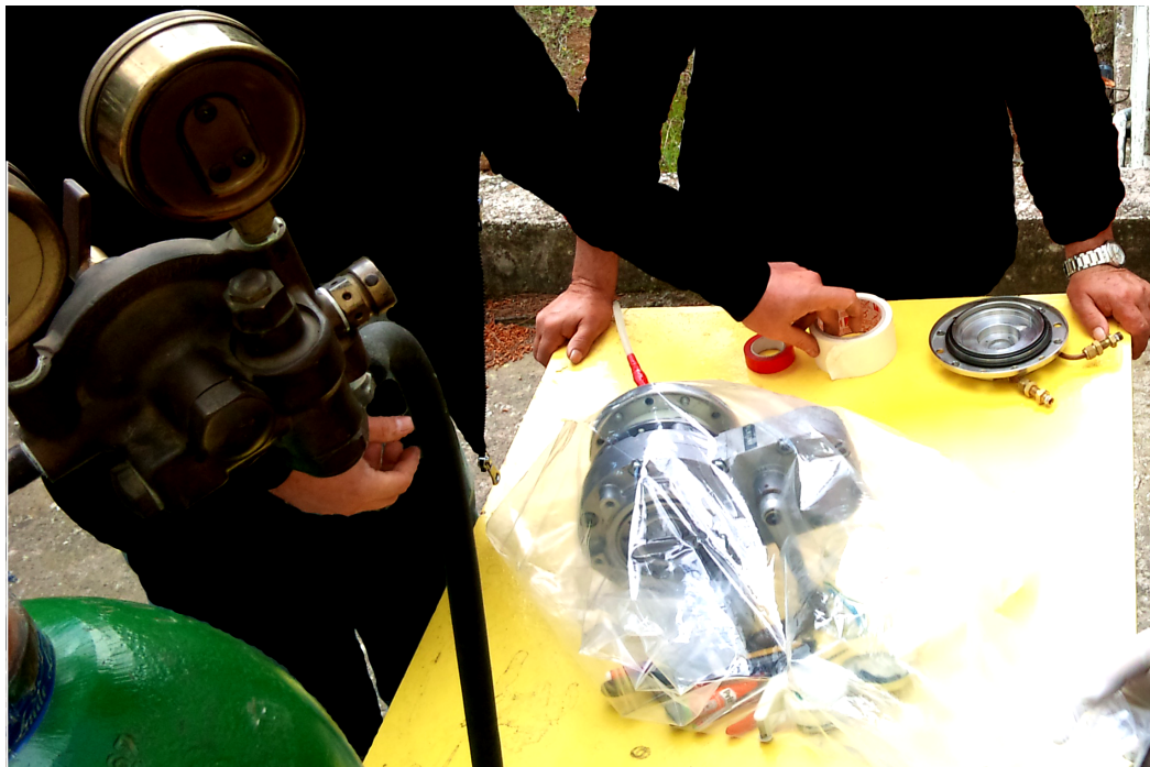
Figure 2.6: The placement of the T target in the flange. The process took place in an airtight isolation bag in an outdoor area due to the high T target activity and its high probability to adhere to air molecules.
