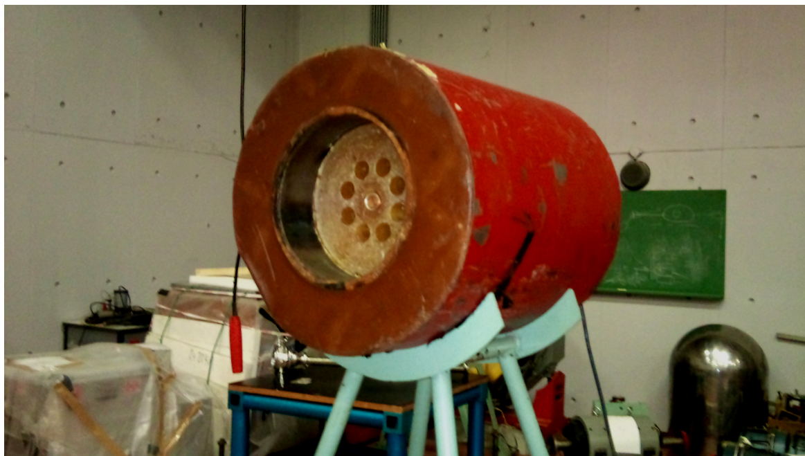
Figure 2.8: \text{BF}_3 detector used for monitoring the neutron beam fluctuations during the irradiations.
