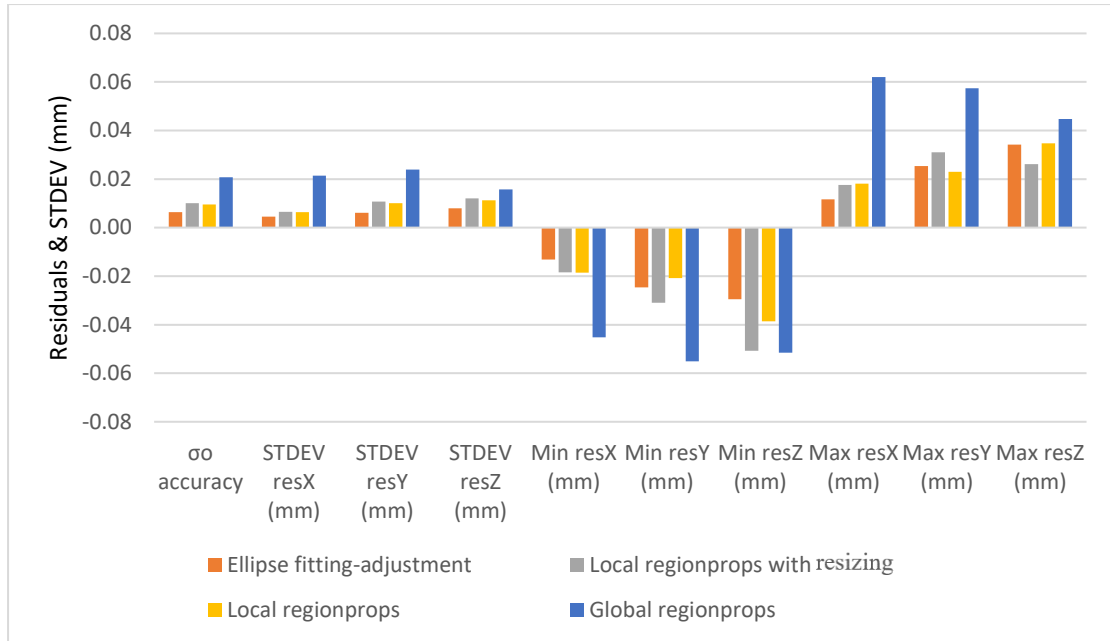
Figure 4.19 Residuals and STDEV of spatial coordinates of targets, measured by the developed algorithms on project 5 after the best fit transformation that uses as reference the spatial coordinates of targets which have been measured by AICON
