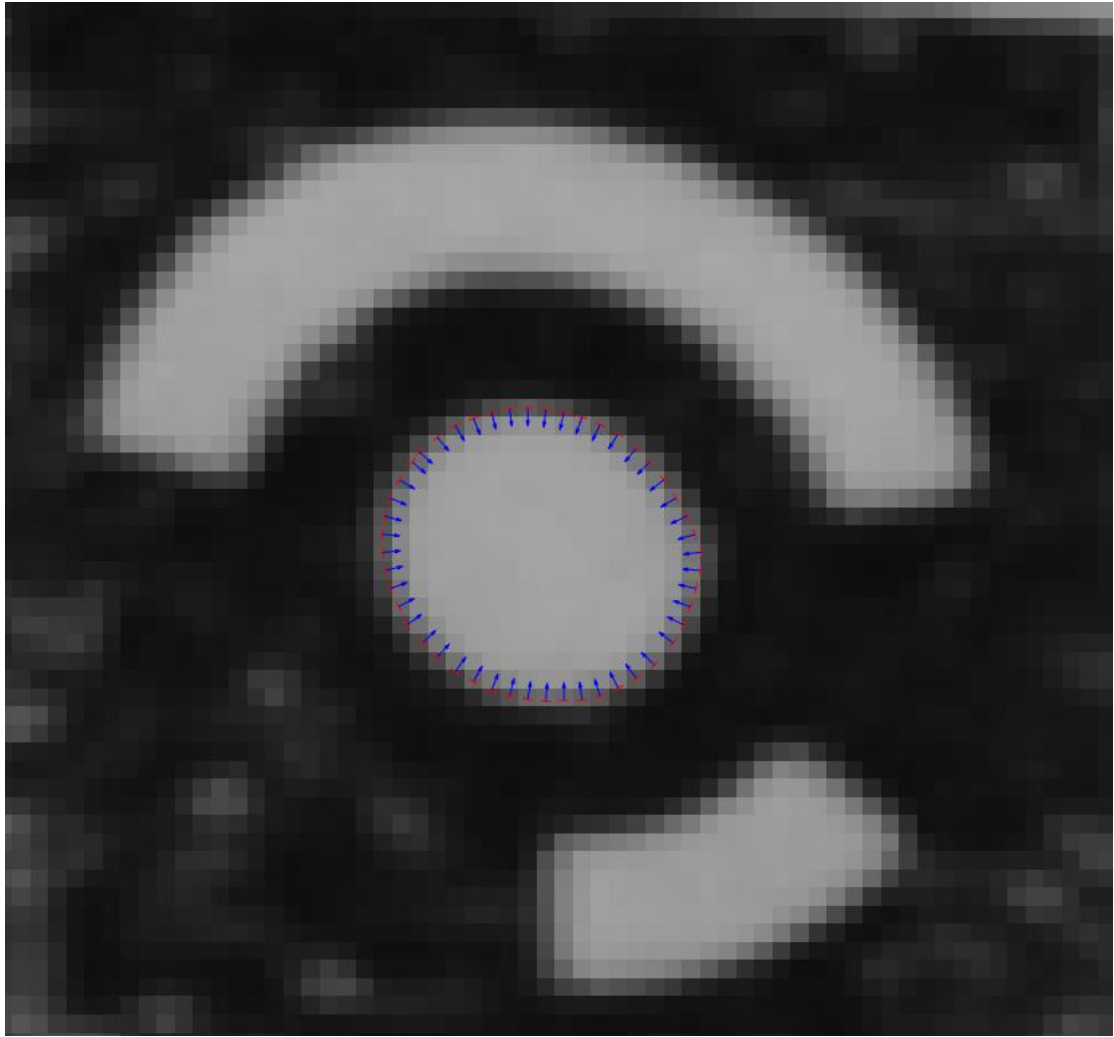
Photo 4.3 Sub-pixel Edge detection on a target
