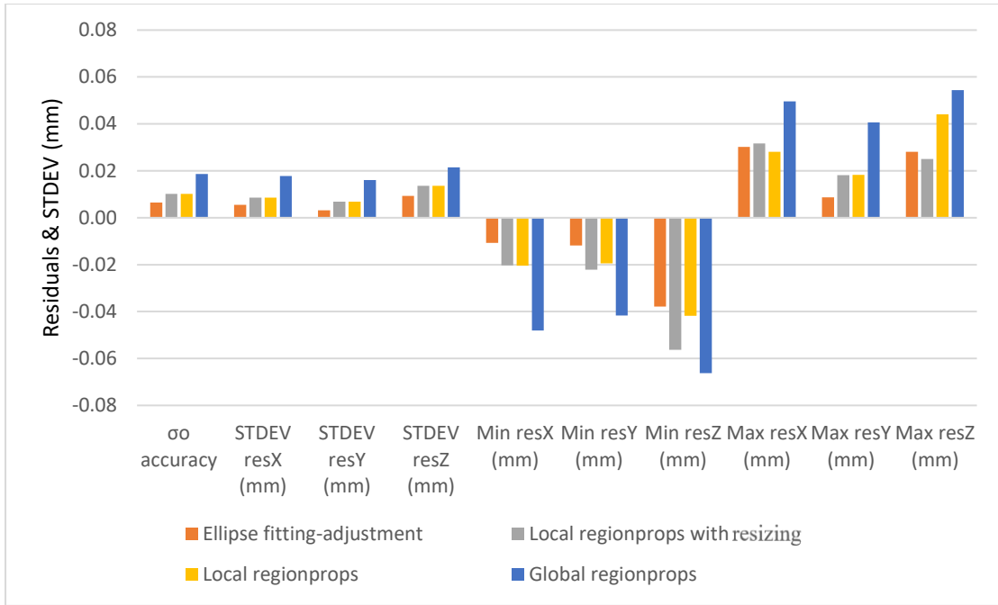
Figure 4.17 Residuals and STDEV of spatial coordinates of targets, measured by the developed algorithms on project 3 after the best fit transformation that uses as reference the spatial coordinates of targets which have been measured by AICON
