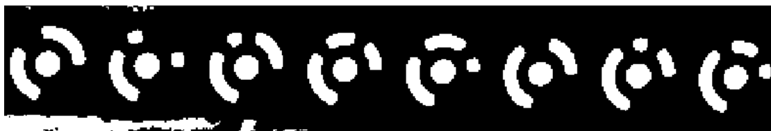
Photo 3.8 Group of targets on binarized image using Otsu's method
