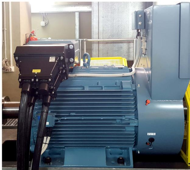
Figure 2.6: ABB Electric Brake 315 kW.
