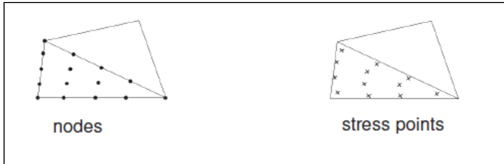
Figure.13 Nodes and stress points in a 15-node triangle element (Plaxis 3D-4-Scientific-1.pdf).
