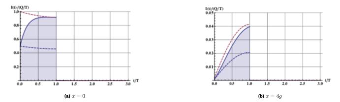
**Figure 31:** Uniform charge movement from for z = 0 to z = g, with  $\epsilon_r = 1, w_x = 4g, b = g, t_0 = 0.1T$ .
