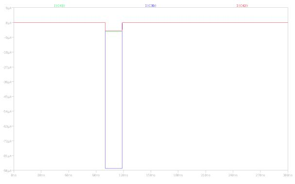
Figure 67: output current for central and neighbor strips
