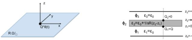
(a) A resistive layer with surface resistance R.
