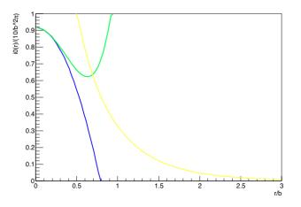
**Figure 19:** Current density  $i_0(r)$  at z = -b. The blue curve represent the second order approximation of (2.74), the green curve the fourth order approximation of (2.74) and the yellow curve the approximation of (2.75).
