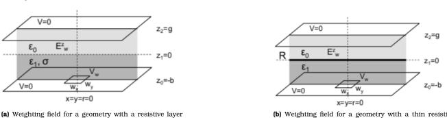
(a) Weighting field for a geometry with a resistive laye having a bulk resistivity of  $\rho = \frac{1}{\sigma}$ .
