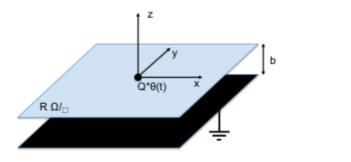
**(a)** A resistive layer with surface resistance R in presence of a ground layer at distance b
