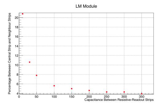
Figure 73: Value of percentage due to capacitance between Resistive-Readout strips.
