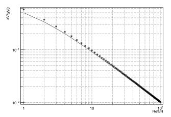
**Figure 28:** Voltage across the center of the resistive plate for a value of f = d/(2a) = 0.01. The dots refer to the exact formula (2.125), the curved line corresponds to the approximation from (2.126).
