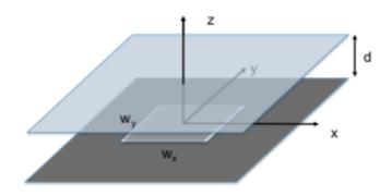
Figure 12: rectangular readout pad
