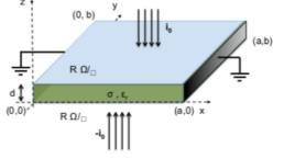
(a) Geometry to define a single resistive layer of thickness d covered by a resistive surface layer of resistance R  $\Omega/$  Square.
