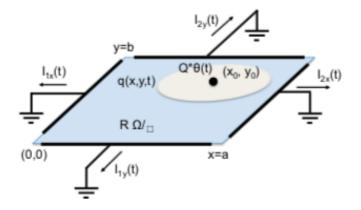
Figure 22: A point charge placed on a resistive layer that is grounded on a rectangle.
