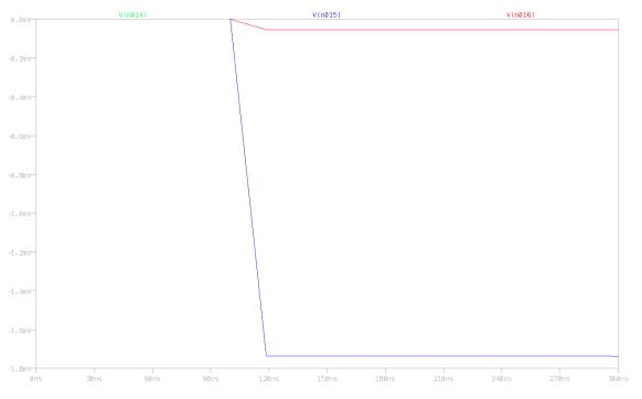
Figure 63: output voltage for central and neighbor strips
