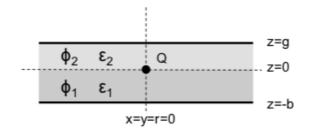
Figure 8: A point charge Q on the boundary between two dielectric layers.
