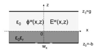
**Figure 17:** Weighting field for a strip electrode of width  $w_x$  and infinity extension.
