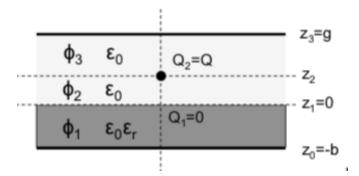
Figure 18: A geometry with three layers and one point charge.
