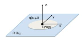
(a) A point charge placed at an infinitely extended resistive layer at t = 0.
