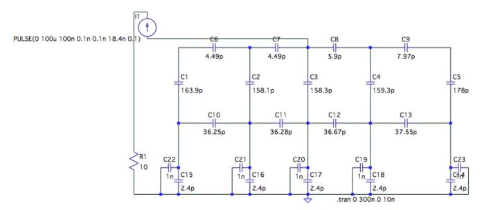
Figure 59: 5 strips SM Module with Spice
