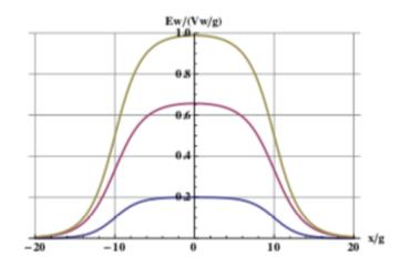
**Figure 16:** Weighting field  $E_z$  at position z = g/2 for b = 4g and  $w_x = 20g$ . The three curves represent  $\epsilon_r = 1$ (bottom),  $\epsilon_r = 8$ (middle),  $\epsilon_r = \infty$ (top).
