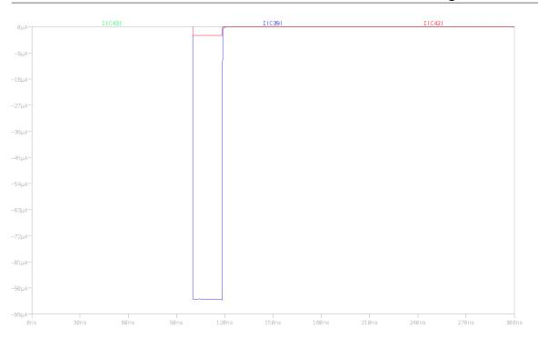
Figure 64: output current for central and neighbor strips
