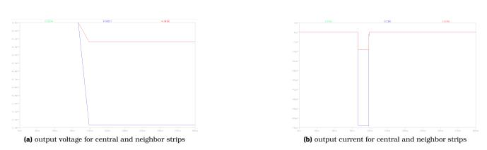
Figure B.6: 250 pf between Readout strips
