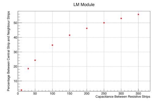
Figure 69: Value of percentage due to capacitance between Resistive strips.
