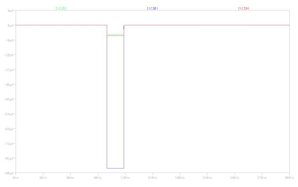
Figure 61: output current for central and neighbor strips
