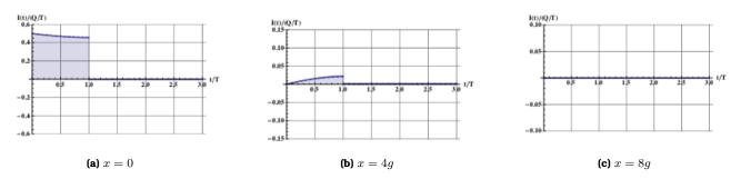
**Figure 33:** Uniform charge movement from for z = 0 to z = g, with  $\epsilon_r = 1, w_x = 4g, b = g, t_0 = T$ .
