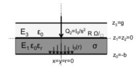
(b) A resistive plate with conductivity  $\sigma$  together with an thin layer of surfave resistivity R\Omega /square and impressed current  $I_0$
