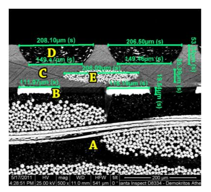
Figure 37: Micromegas Module by microscope
