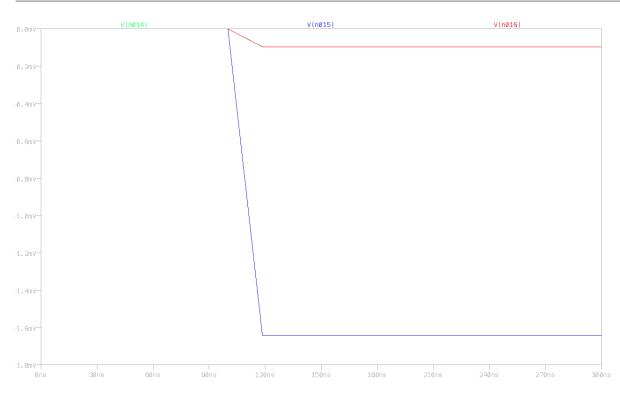
Figure 66: output voltage for central and neighbor strips
