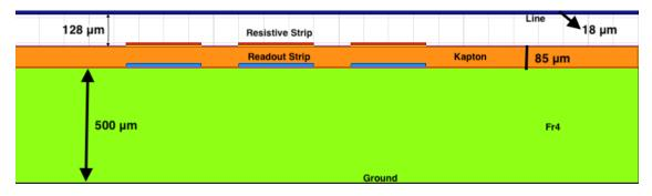
Figure 38: Micromegas Module with 3 Resistive and 3 readout strips.
