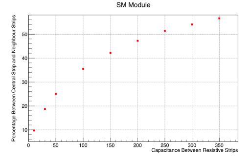
Figure 70: Value of percentage due to capacitance between Resistive strips.
