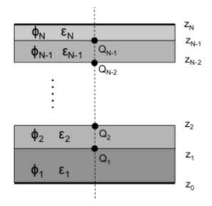
**Figure 13:** A geometry on N dielectric layers enclosed by grounded metallic plates. On the boundary between two layers at r = 0 there are point charges Q.
