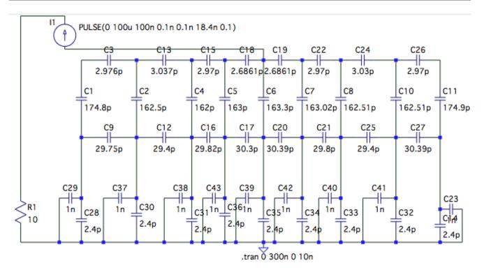
Figure 62: 9 strips LM Module with Spice
