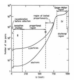
Figure 3: The different regions of gaseous detectors operation with respect to the applied voltage.
