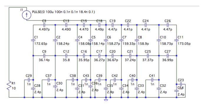
Figure 65: 9 strips SM Module with Spice
