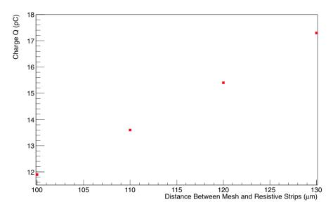
**Figure 10:** Values of charge for different values of distance between mesh and the resistive strips for applied voltage 570 V
