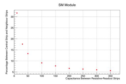
Figure 74: Value of percentage due to capacitance between Resistive-Readout strips.
