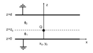
**Figure 11:** A point charge Q in an empty condenser.
