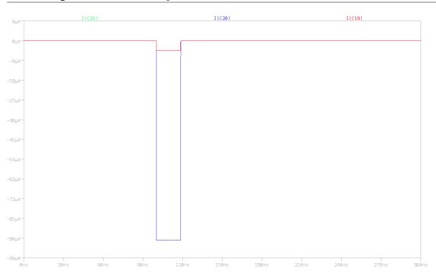
Figure 58: output current for central and neighbor strips
