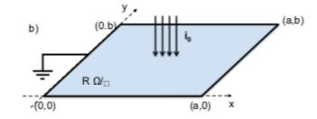
**Figure 26:** Uniform current "impressed" on the resistive layer will result in a potential distribution that depends strongly on the boundary conditions.
