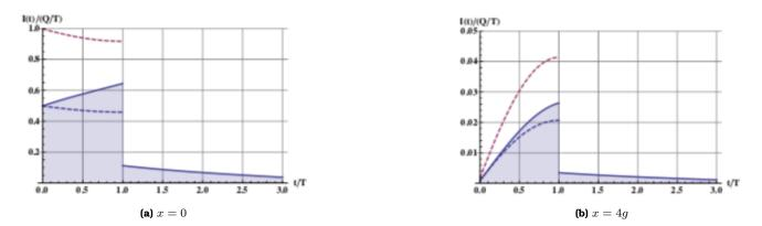
**Figure 30:** Uniform charge movement from for z = 0 to z = g, with  $\epsilon_r = 1, w_x = 4g, b = g, t_0 = T$ .
