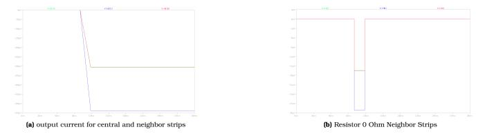
Figure A.18: 350 pf between Resistive strips
