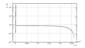
**Figure 6:** Total auxiliary current as a function of time. The peak at the origin lasts for less than 2 ns is due primarily to the electrons movement while after 2 ns the distribution id due to the ion drifting towards the mesh.
