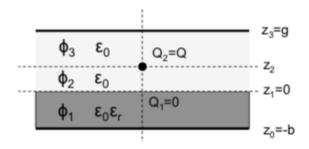
Figure 15: Geometry with three layers and one point charge representing a single gap RPC.
