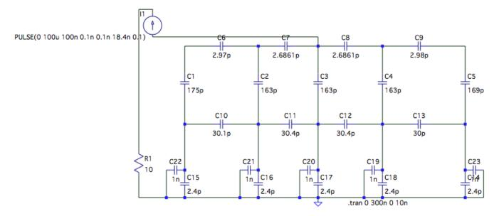
Figure 56: 5 strips LM Module with Spice
