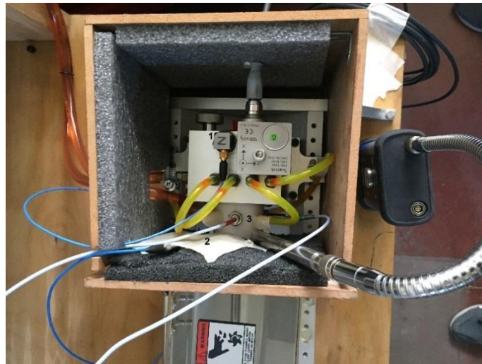
Figure 4.7 Bearing and Soundproof cover mounted with the sensors
