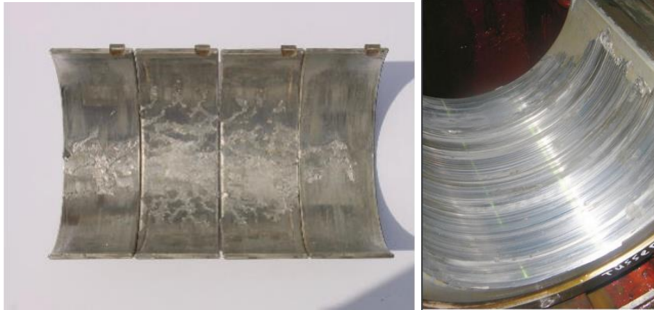
Figure 2.4 Bearing overloading: Metal fatigue (left) and excessive wiping (right)
