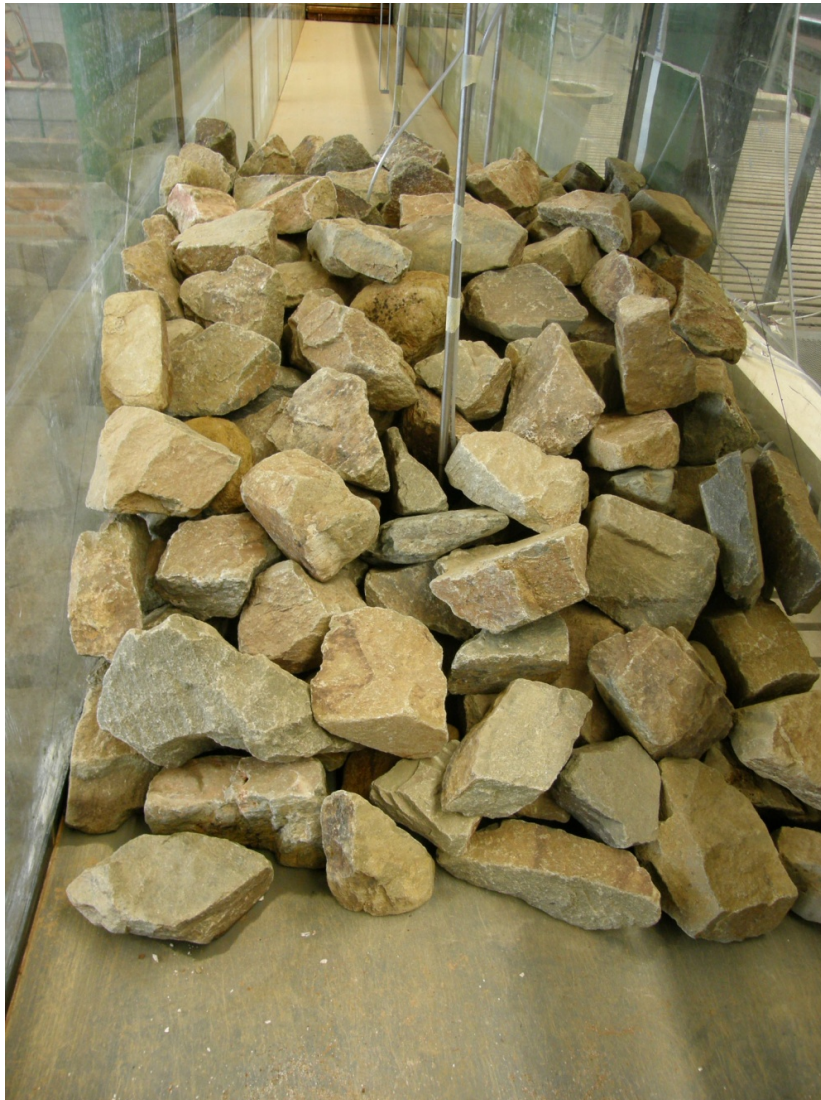
Photo A.1. Breakwater slope close-up
