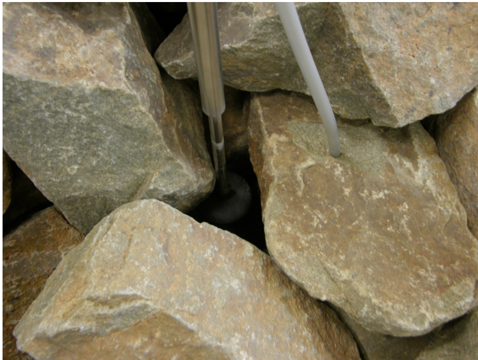
Photo A.3. Velocity transducer and pressure meter close-up
