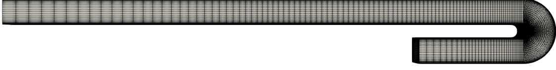
Figure 4.4: Flow through a 3D U-shaped pipe. Computational space and structured grid of the U-shaped with square cross section pipe.
