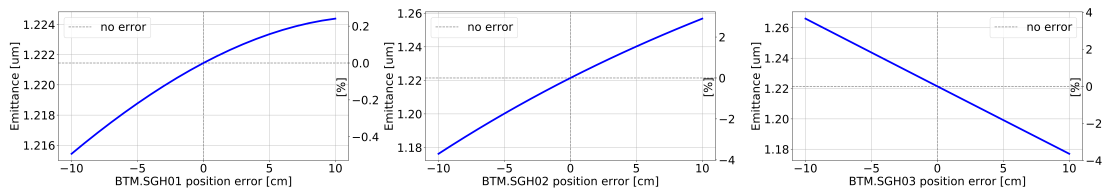
Figure 3.7: Emittance sensitivity on the positions of the SEM grids
