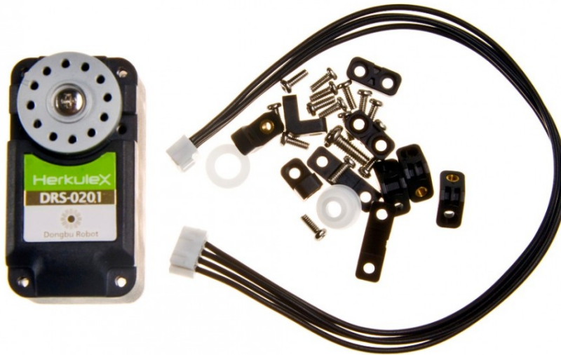
Σχήμα 3.6: HerkuleX DRS-0201 Smart Robot Servo [42]
