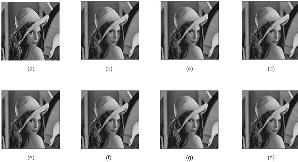
Figure 6.7: Image blurring using the proposed approximate multipliers. (a) Original image (Lena). Image blurring using (b) the accurate multiplier, (c) the PR|_{4,12} design, (d) the PR|_{6,12} design, (e) the PR|_{6,14} design, (f) the PR|_{8,16} design, (g) the PR|_{10,18} design, and (h) the PR|_{10,20} design
