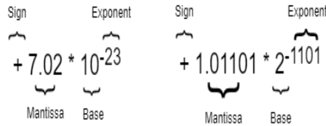
Figure 2.14: A decimal and a binary floating point representation
