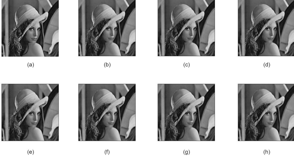
Figure 6.5: Image blurring using the proposed approximate multipliers. (a) Original image (Lena). Image blurring using (b) the accurate multiplier, (c) the PR|_{0,2} design, (d) the PR|_{1,0} design, (e) the PR|_{1,4} design, (f) the PR|_{3,4} design, (g) the PR|_{3,6} design, and (h) the PR|_{4,6} design
