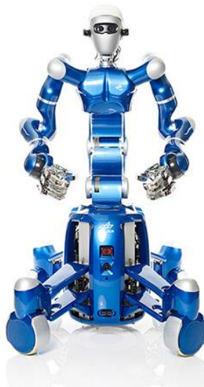
Figure 1-4: Overview of the Justin mobile platform system [9].
