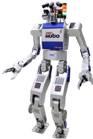
Figure 1-5: DRC-Hubo+ is a versatile humanoid that won first place at the DARPA Robotics Challenge in 2015. The robot can use tools, open doors, and even drive a vehicle. It can transform itself from a walking biped to a wheeled machine [19].
