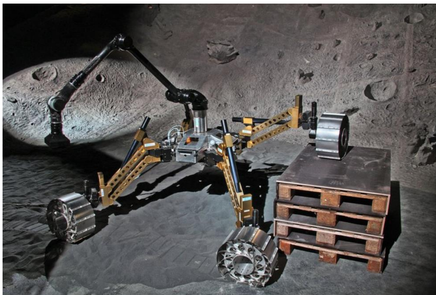
Figure 1-2: Sherpa stepping onto a high obstacle. The manipulator was used to support the rover while lifting the wheel onto the obstacle [5].
