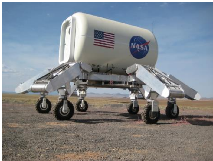
Figure 1-8: Tri-ATHLETE robot, a six-legged robot developed at the NASA's Jet Propulsion Laboratory in southern California [11].
