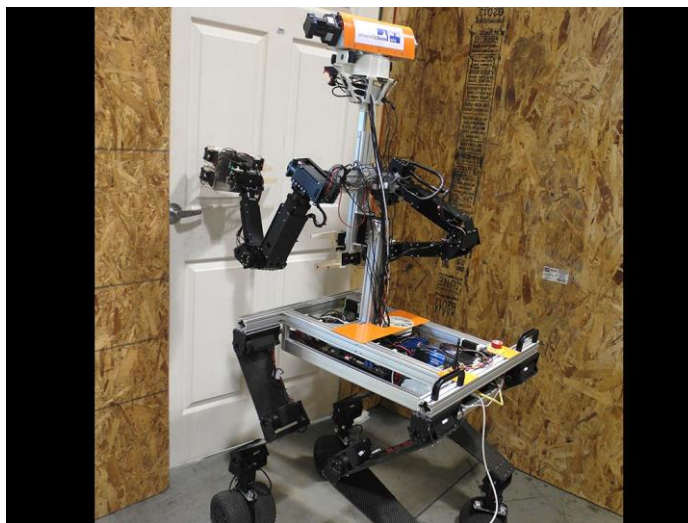
Figure 1-6: Momaro is a mobile robot that can carry out sensing and manipulation tasks in disaster sites and other harsh environments. It was designed to compete in the DARPA Robotics Challenge, coming in fourth place [16].
