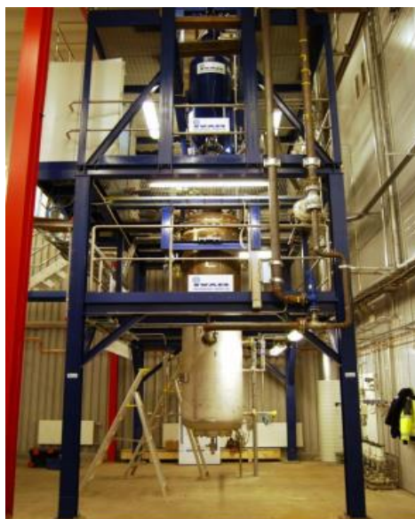
Figure 3-9: Depiction of the pilot-scale 1 MW th biomass-fueled PEFG unit at ETC.
