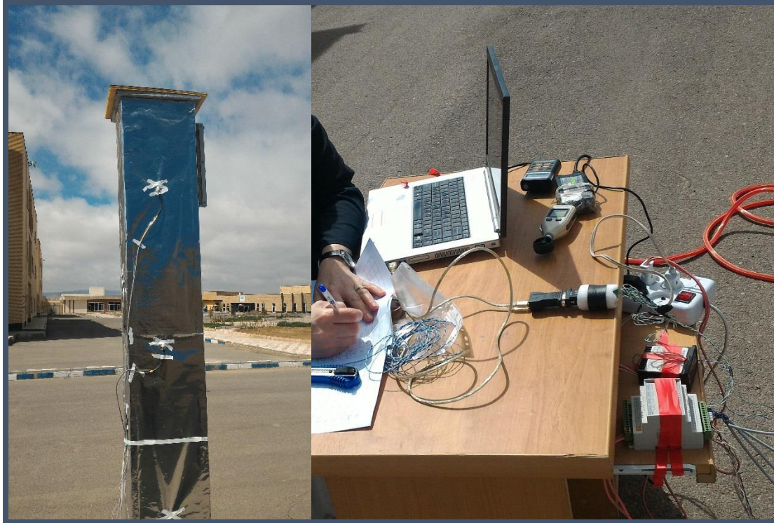
Figure 24. The sensors were connected to a personal computer by means of a temperature transmitter
