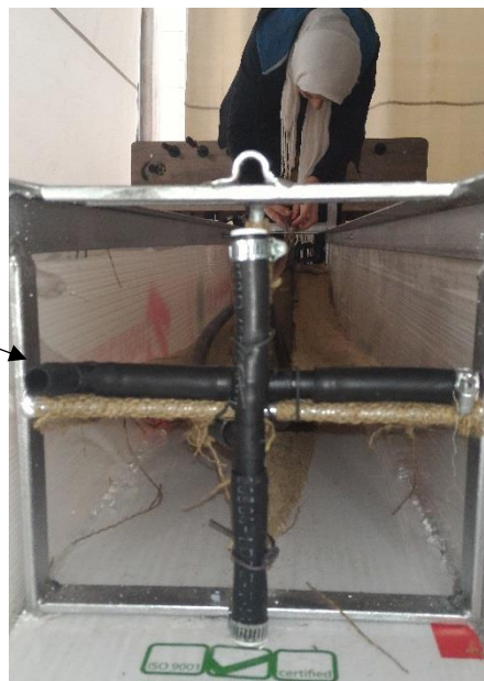
Figure 21. Drip tubing mounted on blades
