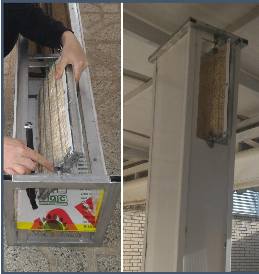
Figure 20. Constructed pad is installed in prototype wind catcher
