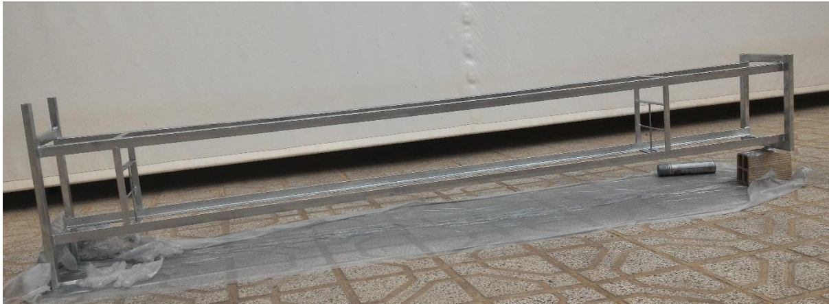
Figure 18. The metal structure of the model before installing the wall
