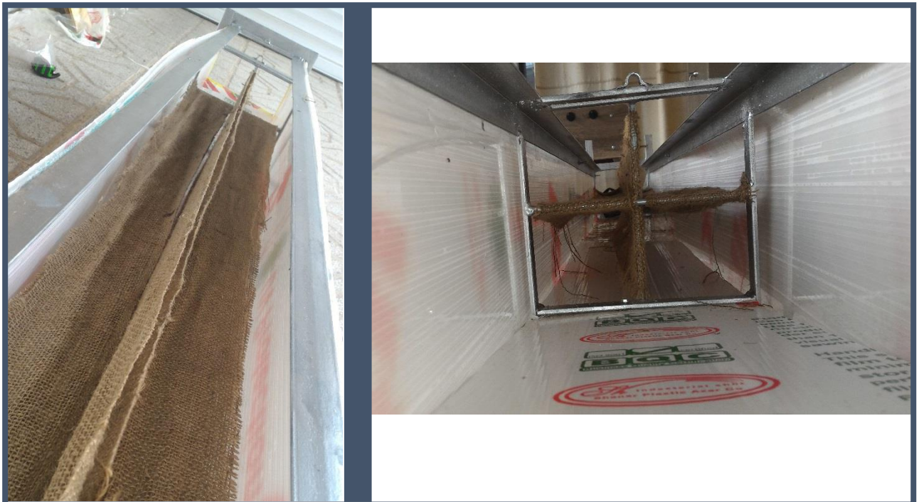
Figure 19. The blade section with plus shape and gunny screens
