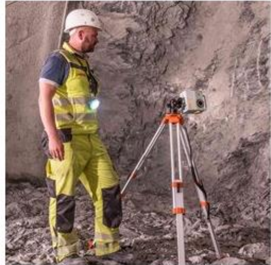
Figure 2.6: Tunnel profilemeter (source: Ryu et.al. 2008; www.dibit.at).
