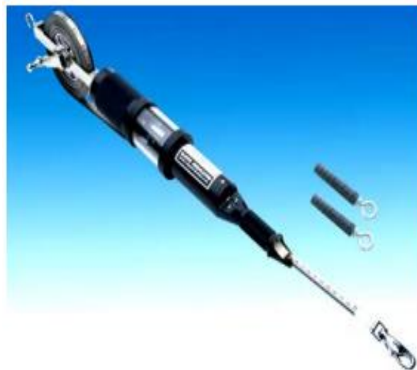
Figure 2.4: Digital tape extensometer and its installation in measuring tunnel convergence.
