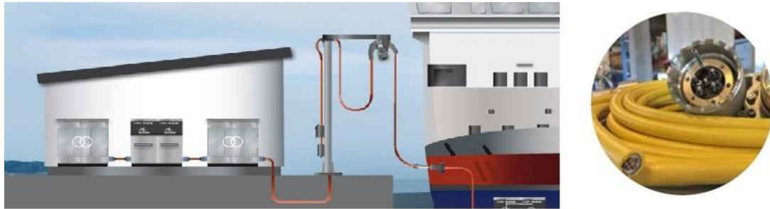
Figure 2.13 – CI cable arrangement option and a closer look at an installation cable
