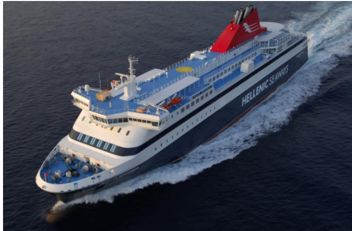
Figure 1-3. Fast displacement ferry Nissos Mykonos operates at a service speed of 26 knots, corresponding to a Froude number of 0.38. Source: Attica Group.
