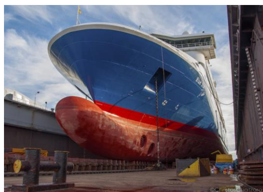
Figure 1-5. Bulbous bow of modern ro-pax ferry. Source: www.shipfriends.gr .
