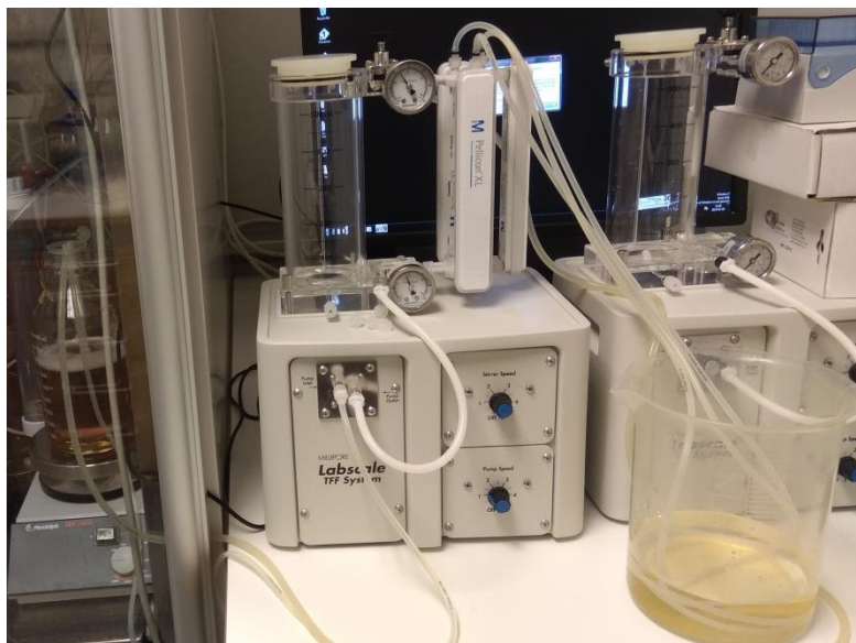
Figure 2.5. Ultrafiltration system that was used.
