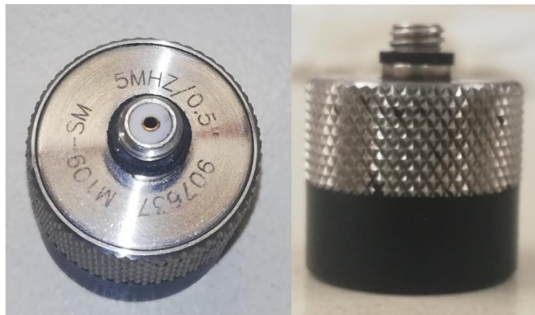
Figure 4.5 Microscan transducer M109-SM, 5 MHz.
