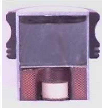
Figure 2.18 Piezoelectric ceramic element inside a cutten transducer.
