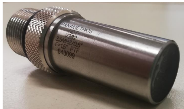
Figure 4.7 Immersion transducer V382-SU, 3.5 MHz.
