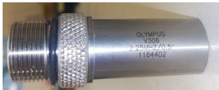
Figure 4.6 Immersion transducer V306-SU, 2.25 MHz.
