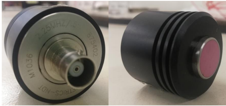
Figure 4.4 Microscan transducer M1036, 2.25 MHz.
