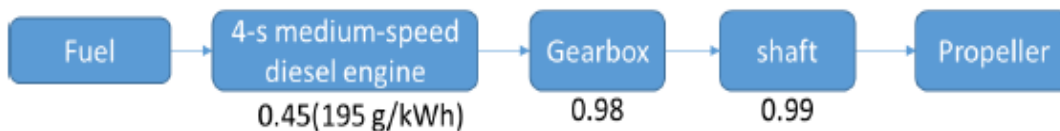
Typical diesel-mechanical propulsion chain
