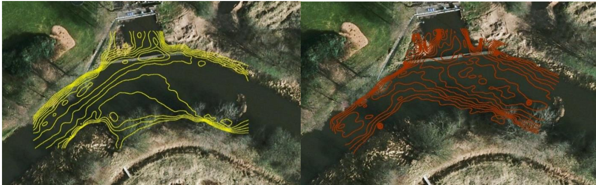
Figure 2: Bathymetry and velocity contour lines of the case study area from left to right respectively.
