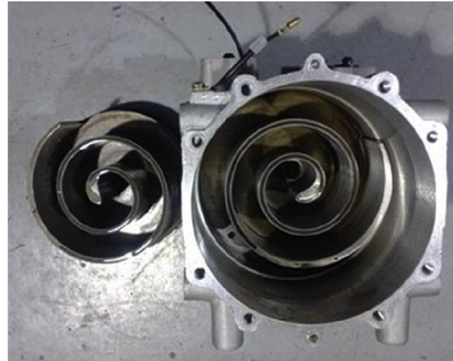
Figure 2.13: Operating principle & the scroll wraps of a typical helical expander (scroll). [42]
