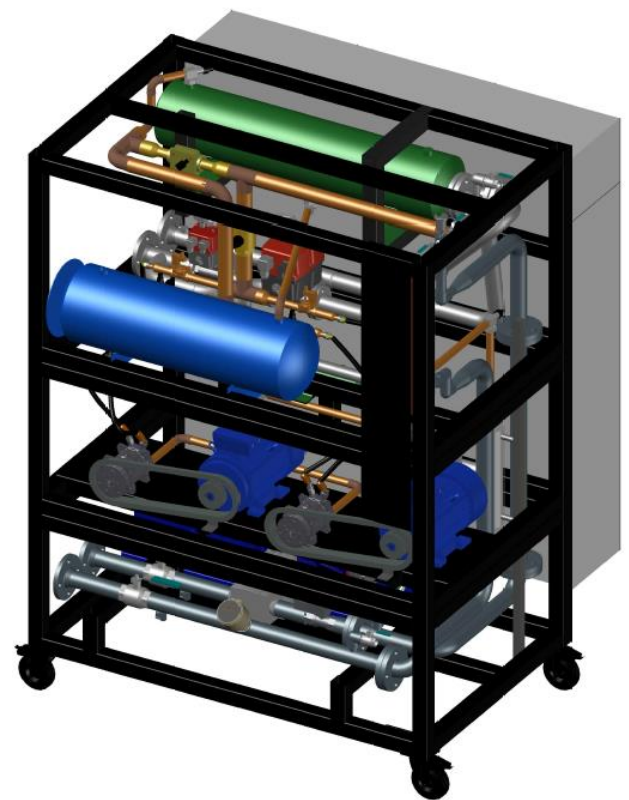
Figure 4.13: Final arrangement of on board marine ORC prototype & 3D AutoCAD drawing.
