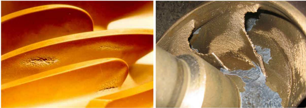
Figure I.3 Typical cavitation damage on the blades of centrifugal pumps (Brennen, 2014; Kamiel, 2015).
