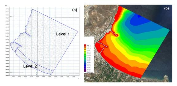
Figure 5-11. (a) Mesh with triangles using two levels for the inner model domain. (b) The inner model domain showing the bathymetry of the examined area.
