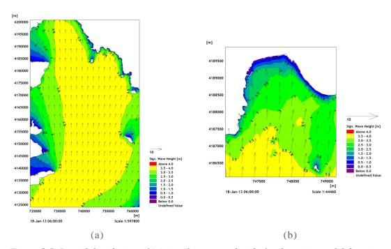
Figure 5-5. Spatial distribution of (a) significant wave height for the entire model domain and (b) for Varkiza bay at a specific time step of the simulation.
