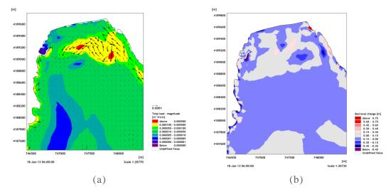
Figure 5-6. Spatial distribution of (a) seabed level change and (b) total magnitude of sediment transport for Varkiza bay at a specific time step of the simulation.
