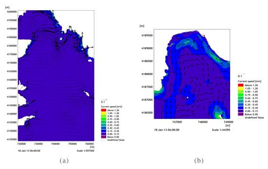
Figure 5-4. Spatial distribution of (a) current speed and current direction for the entire model domain and (b) for Varkiza bay at a specific time step of the simulation.
