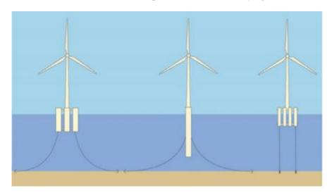
Figure 3-2. Floating wind turbine support structures: (left) semi-submersible structure; (middle) spar-type structure; and (right) tension leg platform (Wu et al., 2019).
