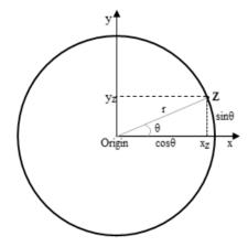
Figure A-1. Graphical representation of rectangular and orthogonal coordinate systems.
