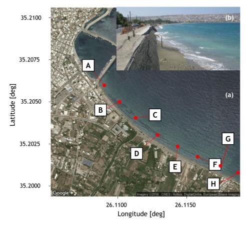
Figure 5-15. (a) Map of the examined area (from Google Earth) indicating the locations for the estimation of seabed level based on the proposed methodology at Sitia beach. (b) Photo near location G indicating erosion problem.
