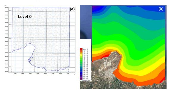
Figure 5-10. (a) Mesh with triangles for the outer model. (b) The bathymetry of the outer model domain.
