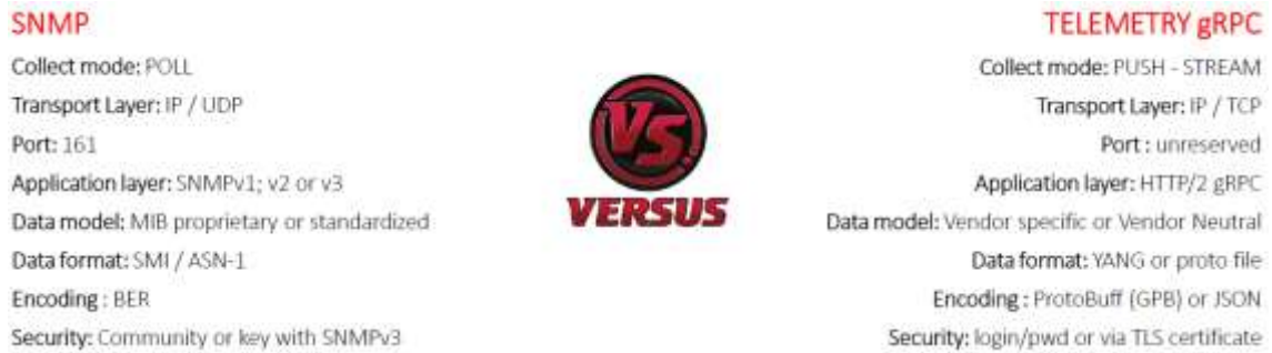
Figure 2.11 SNMP vs Telemetry 2
