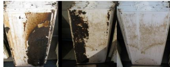
Photograph 3: Examples of severe sludge caking observed
