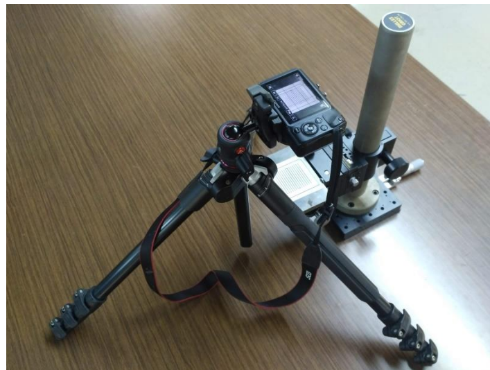
Fig. 6-2 Adjustable platform, camera and tripod configuration for specimen measurement.
