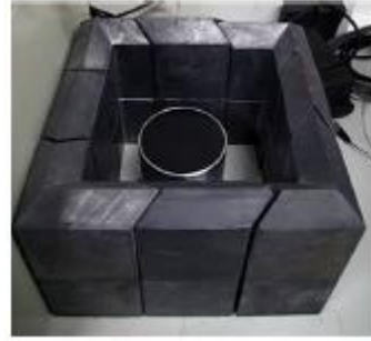
b) The shielding of HCMR's detector
