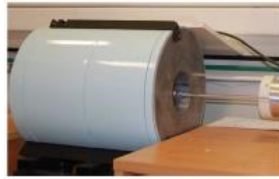
d) The shielding of NTUA's detector
