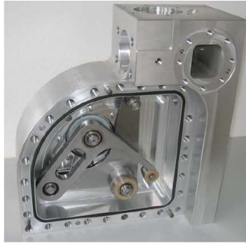
Figure 2.8. The Carlsen crank mechanism of the Dortmund University hybrid Stirling-Vuilleumier machine. Image obtained from [86].
