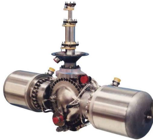
Figure 2.6. The Hughes Aircraft Company Hi-Cap Vuilleumier cryocooler. The two big cylinders enclose the opposing displacers and the 3 (bronze colored) flanges at the top indicate the 3 cold stages. Image obtained from [47].
