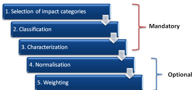
Figure 73: LCIA steps according to ISO standards
