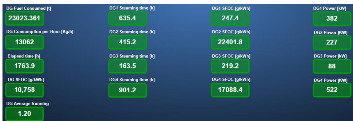
Figure 96: Open sea cargo ship. Fuel consumption at port (source: RINA)
