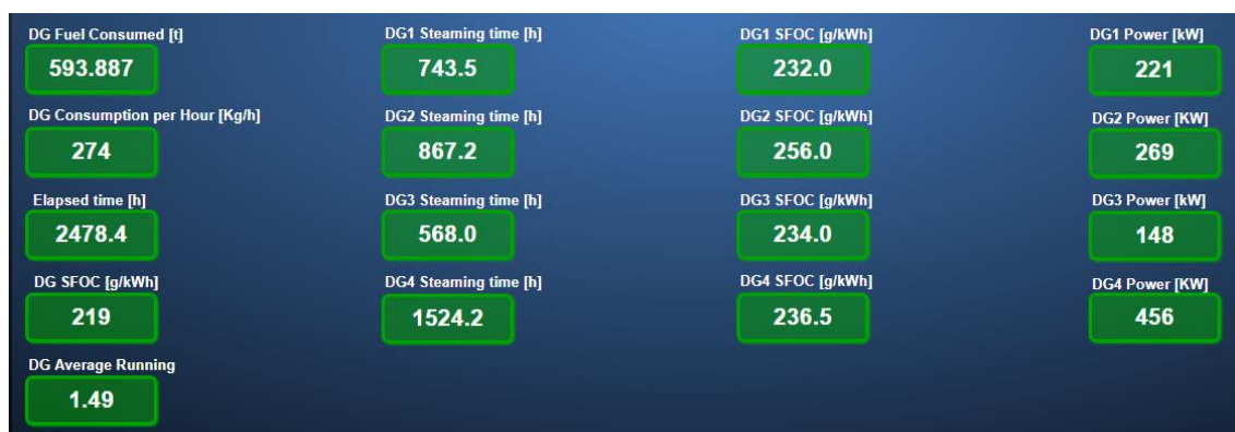
Figure 95: Fuel consumption data at port of short sea shipping container ship (source: RINA)
