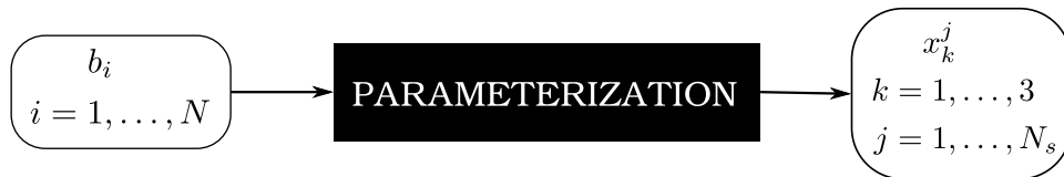
Figure 4.1: Shape parameterization may be considered as a process linking the N design variables to the coordinates of the N_s nodes.
