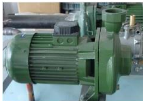
Figure 3.15 Centrifugal pump K 18/500 T, DAB company
