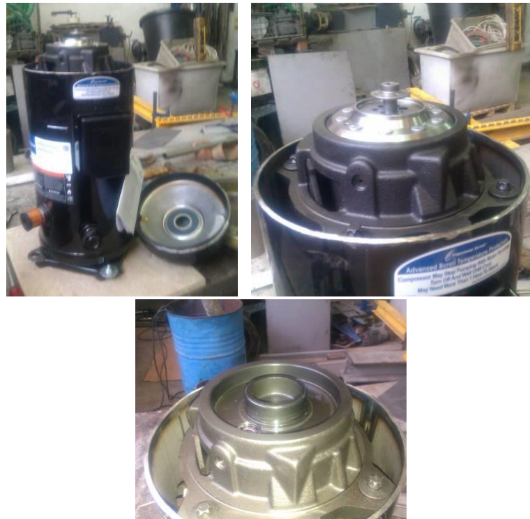
Figure 3.25 Cutting and removal of the scroll compressor's upper part
