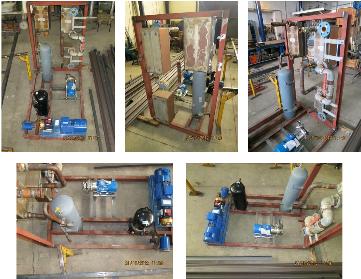
Figure 3.37 Several views of the ORC engine where the frame and several components (heat exchangers, organic fluid pump, scroll expander, receiver, heat cycle pump) are observed
