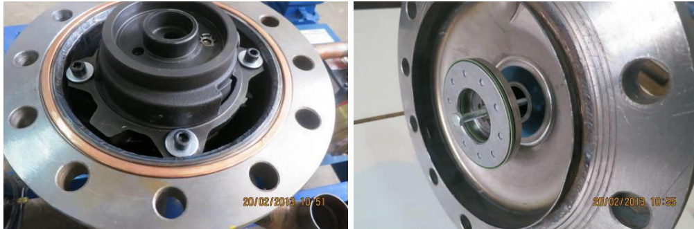
Figure 3.30 Small hole (left) and adjustable thread on the cap of the scroll compressor (right)
