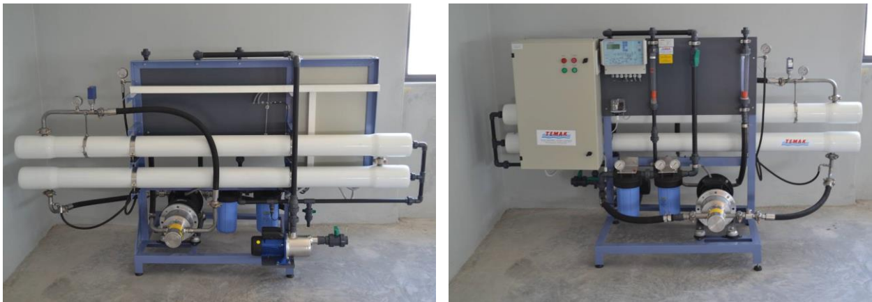
Figure 3.61 Back and front view of the RO sub- unit to be installed in the laboratory
