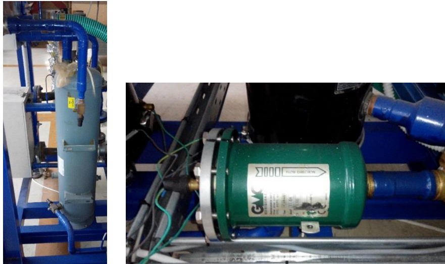
Figure 3.16 Receiver vessel and filter of the organic fluid
