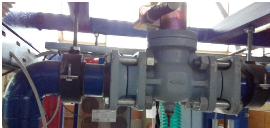
Figure 3.33 Electro valve for the single and two- stages interval
