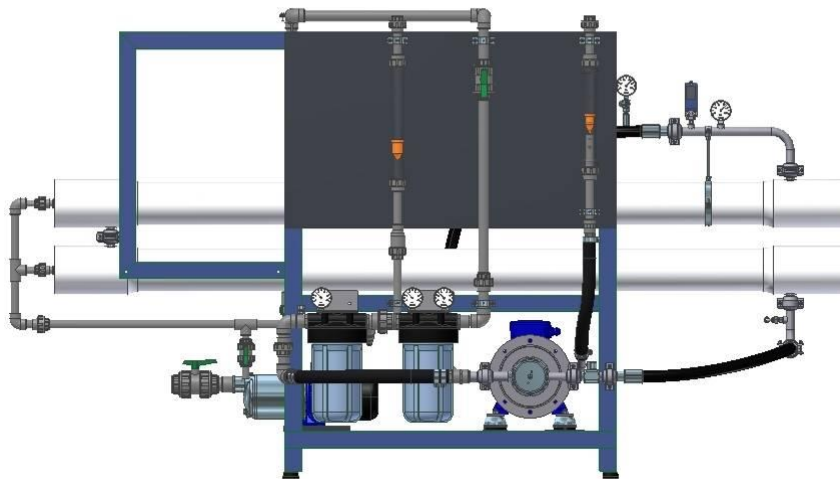
Figure 3.59 Flexible pipes at the inlet and outlet of the HP pump
