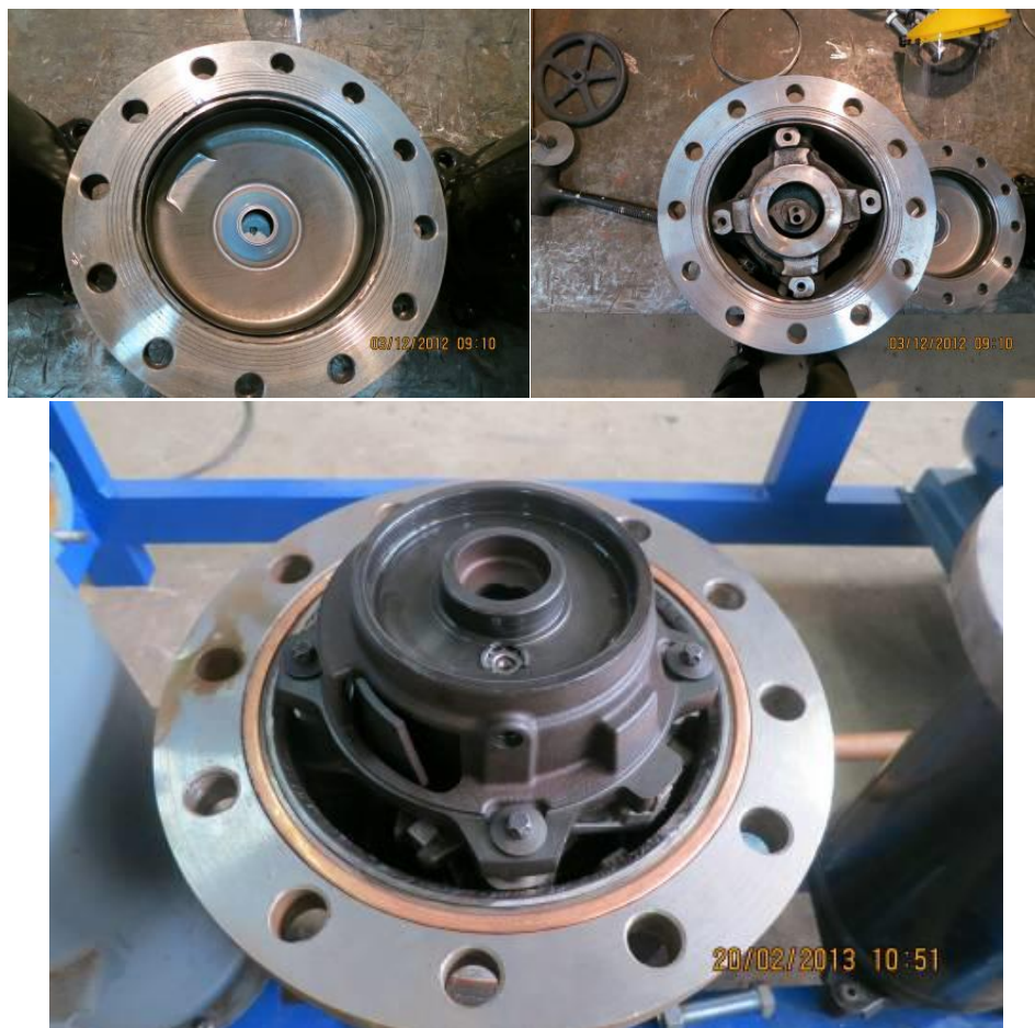
Figure 3.26 Scroll compressor's internal part
