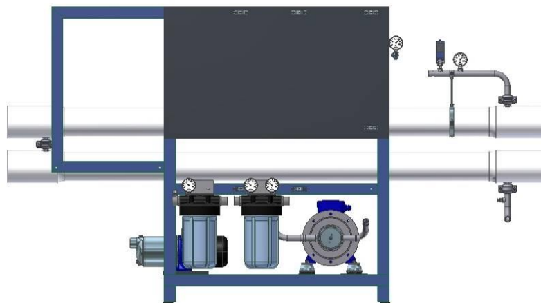
Figure 3.57 Basic equipment placement
