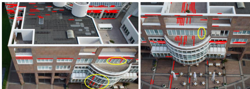
Figure 6-6. Automatically detected horizontal line segments superimposed in magnified parts of images of UAV Dataset 2 , among which the wrongly identified horizontal line segments are marked by yellow ellipses
