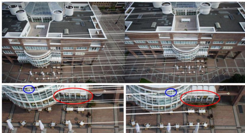
Figure 7-20. Image matching results between a pair of UAV images using SURF; top: detected correspondences; bottom: details illustrating remaining outliers, marked with red and blue ellipses
