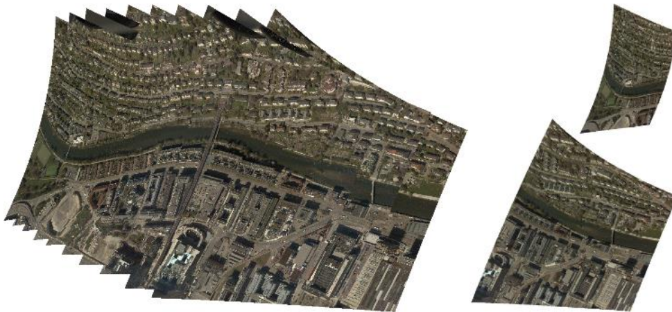
Figure 4-6. Left: a strip of rectified georeferenced oblique aerial imagery from the RCD 30 Oblique Penta Dataset after the application of a second order polynomial transformation; right: the first (bottom) and last (top) rectified images of this strip, indicating changes in ground footprint
