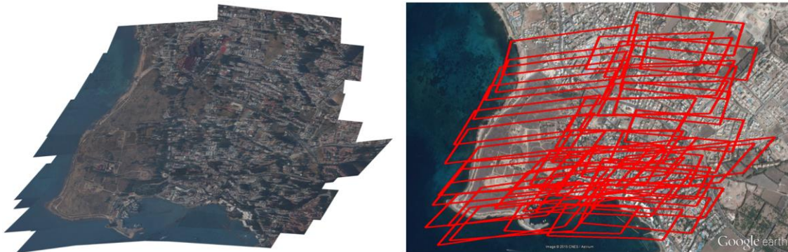
Figure 4-8. Left: insertion of the rectified georeferenced oblique aerial imagery of the Canon EOS-1Ds Dataset in a GIS environment (affine transformation used); right: superimposition of the footprints of the Canon EOS-1Ds Dataset on Google Earth imagery
