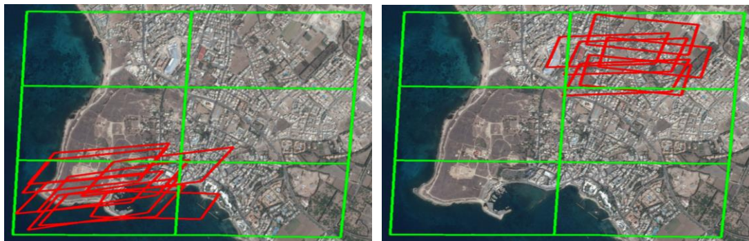
Figure 4-9. Subdivision of the Canon EOS-1Ds Dataset into groups of images based on their footprints: the user draws the outer green polygon in Google Earth environment; this polygon is automatically divided into cells and each image footprint (in red) is placed in the appropriate cell, using the developed tool
