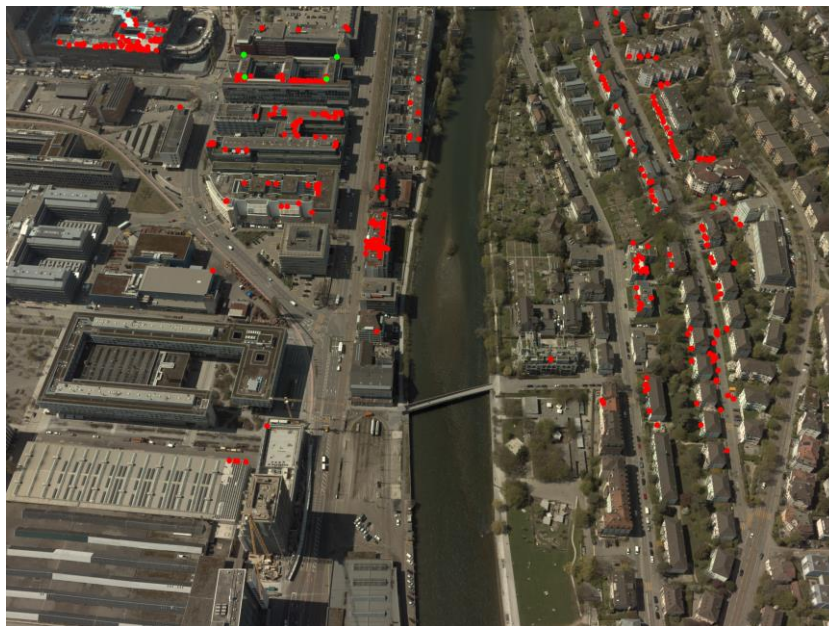
Figure 7-12. Automatically detected coplanar feature points in img_1 of RCD 30 datasets (shown in red) that lie on the plane of the four manually measured coplanar GCPs (shown in green)
