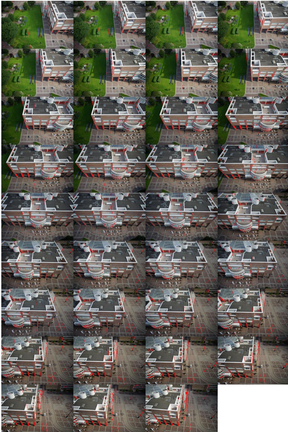
Figure 6-9. Automatically detected vertical line segments in the images of UAV Dataset 2
