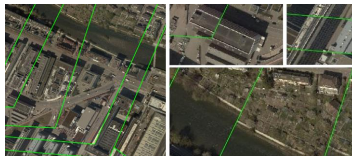
Figure 4-5. Details of the rectified georeferenced images of the RCD30 Oblique Penta Dataset with the borders of their footprints superimposed on them in green (homography transformation used)
