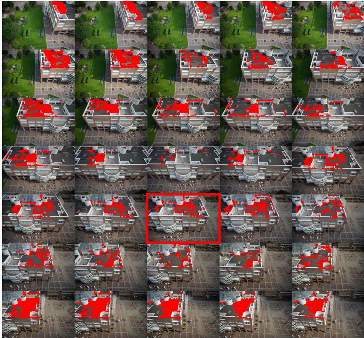
Figure 5-9. Automatically detected coplanar feature points in the images of UAV Dataset 2 ; img_1 is marked by a red outline
