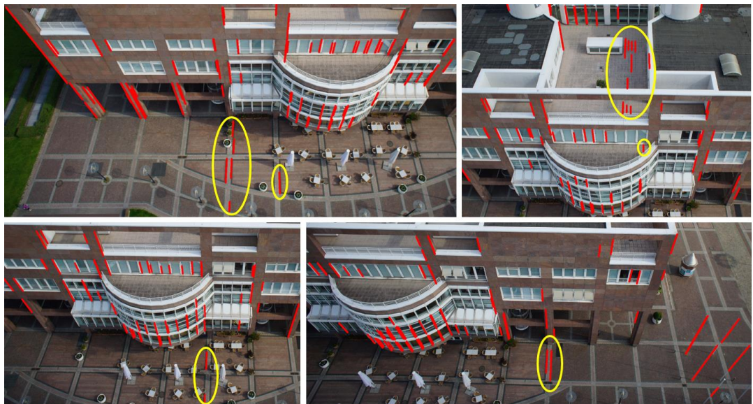
Figure 6-8. Automatically detected vertical line segments superimposed in magnified parts of images of UAV Dataset 2, among which the wrongly identified vertical line segments are marked by yellow ellipses
