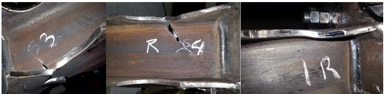
Fig. 3.23 Test T5, crack propagation on specimens (a) S3, (b) S4 (c) crack initiation on S1
