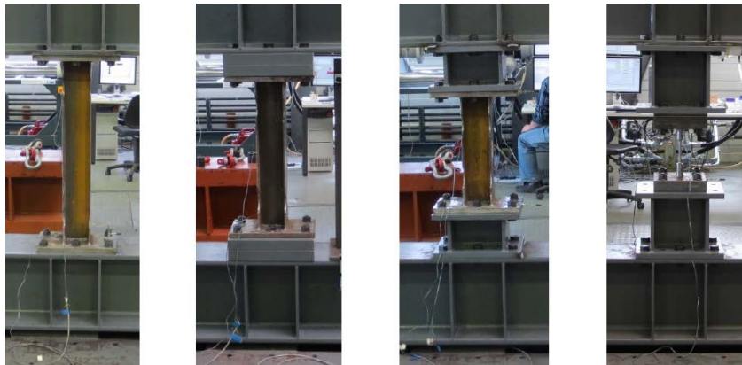
Fig. 3.39 Mounting of FUSEIS components with different lengths
