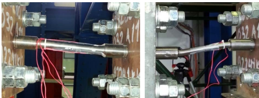
Fig. 3.44 Pins' deformation (a) link S1 (b) link S4
