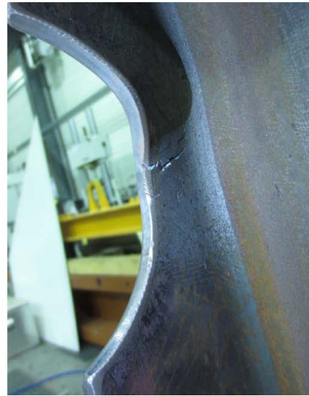
Fig. 3.40 Test CT4 (HEA fuse): response curve and crack initiation (Feldmann et al. 2017)
