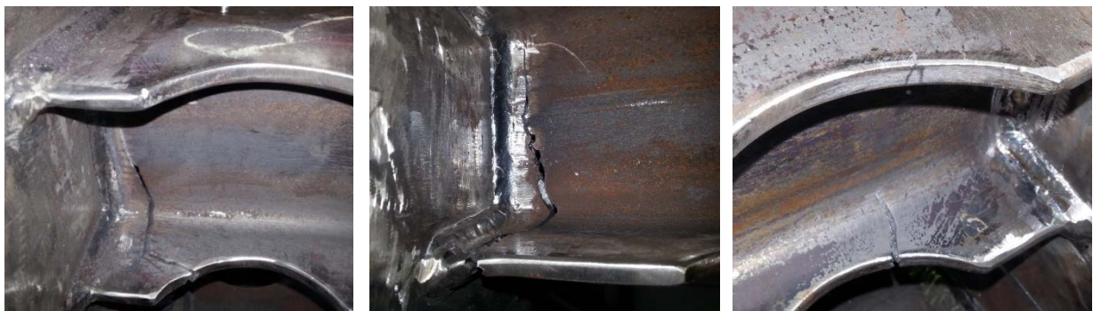
Fig. 3.22 Test T4, crack propagation on specimens: (a) S3, (b) S4, (c) S1
