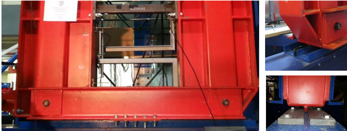
Fig. 3.6 (a) UPN beams providing “diaphragm” action and (b) steel members as “leaders” to prevent out-of-plane displacements
