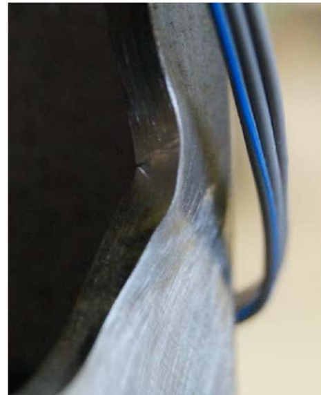
Fig. 3.41 Test CT8 (SHS fuse): response curve and crack initiation (Feldmann et al. 2017)
