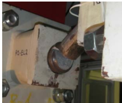
Fig. 3.58 Fracture of specimen in system test M4 (Dimakogianni 2017)
