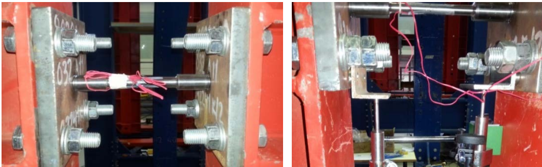
Fig. 3.11 Strain gages at middle of pin's reduced section and LVDTs for measuring plate slippage
