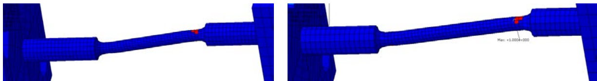
Fig. 4.25 Fracture initiation (red) in links S5 and S4
