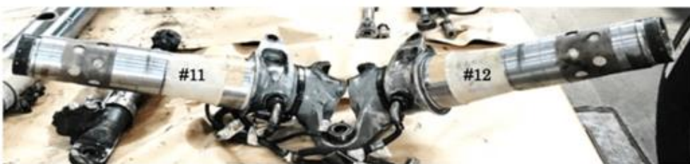
R-MLG AFT axle (Rear View)
