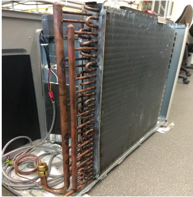
Figure 5.4: The condenser used in the experiments at the University of Bayreuth.
