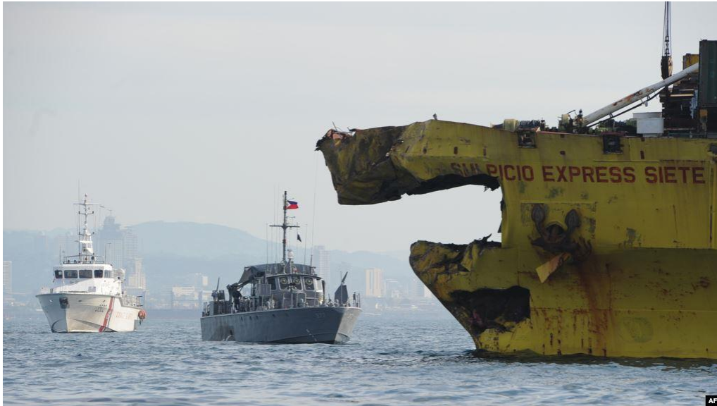
Figure 5.4: The cargo ship “Sulpicio Express Siete” after the collision (Radio Free Europe/Radio Liberty, 2013)
