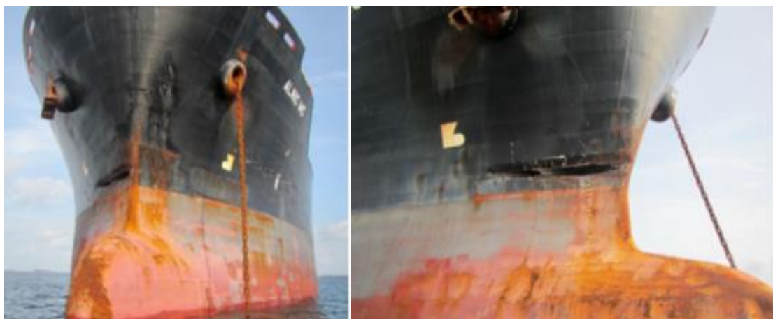
Figure 5.3: The “Alnic MC” oil tanker after the collision casualty (National Transportation Safety Board, 2017)
