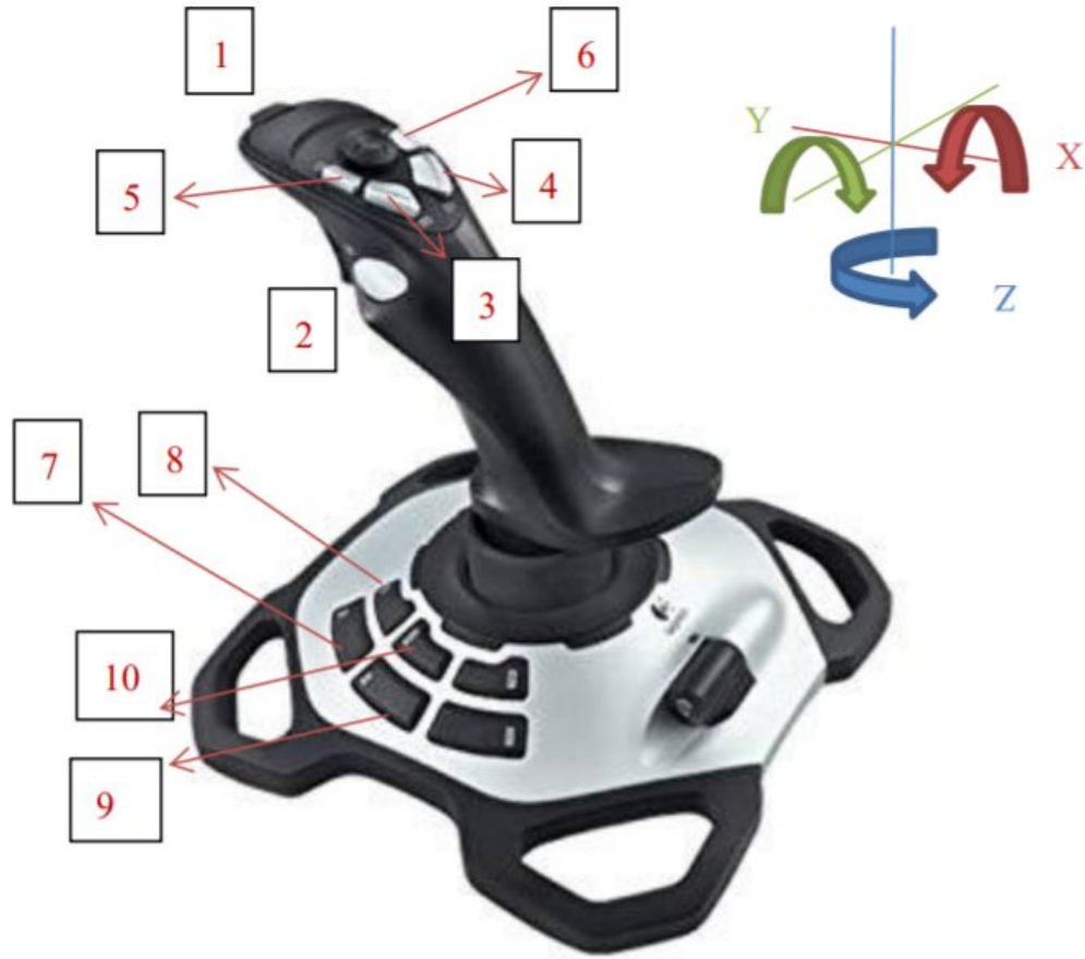
Figure 23: Joystick with numbered buttons and axis of rotation
