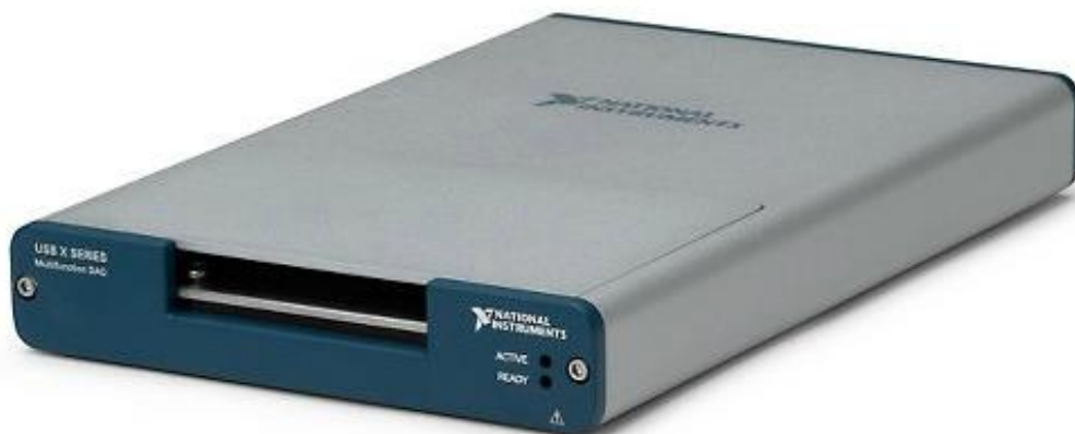
Figure 2-5. Data Acquisition unit NI USB-6351 by National Instruments.
