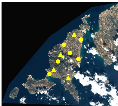
Figure 2. Ground control points and check points used for Pleiades 1B data
