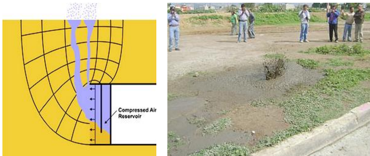
Figure 10: Schematic presentation of face blow-out (left); Capture of the phenomenon from the surface (right) (www.facesupport.org; Redmond & Romero, 2011)
