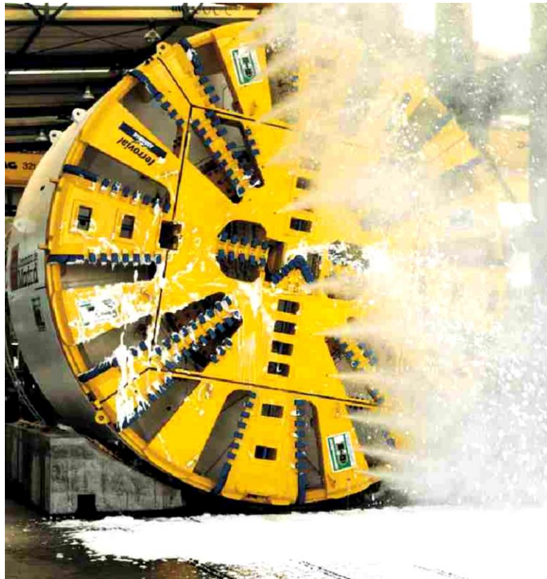
Figure 16: Testing of foam injection in an EPBM cutterhead (Kavvadas M. et al., 2013)
